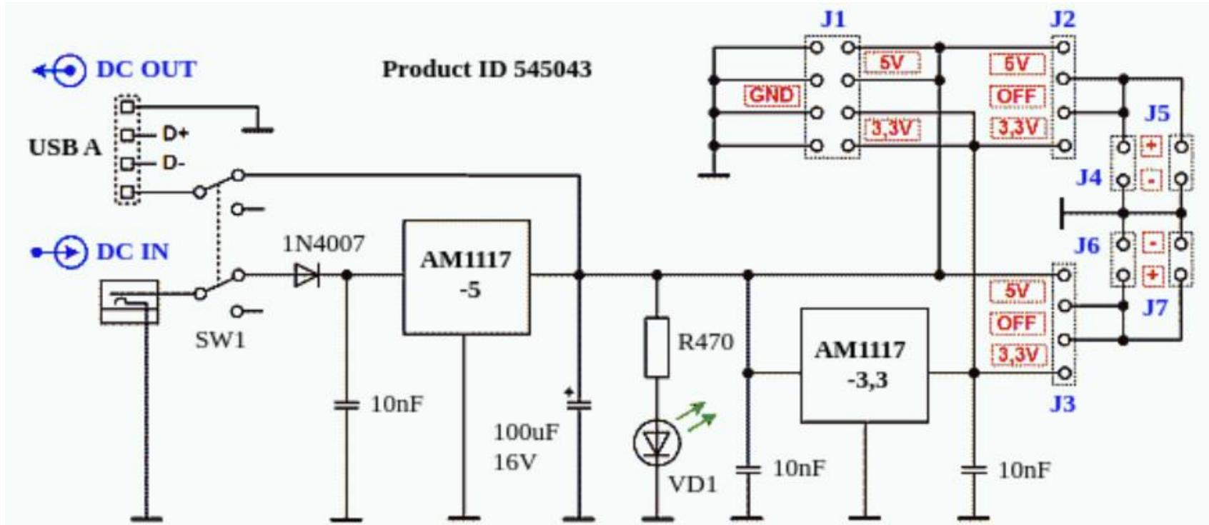
Input voltage (DC IN): 6,5 - 12V, DC barrel jack 5,5mm x 2,1mm.
